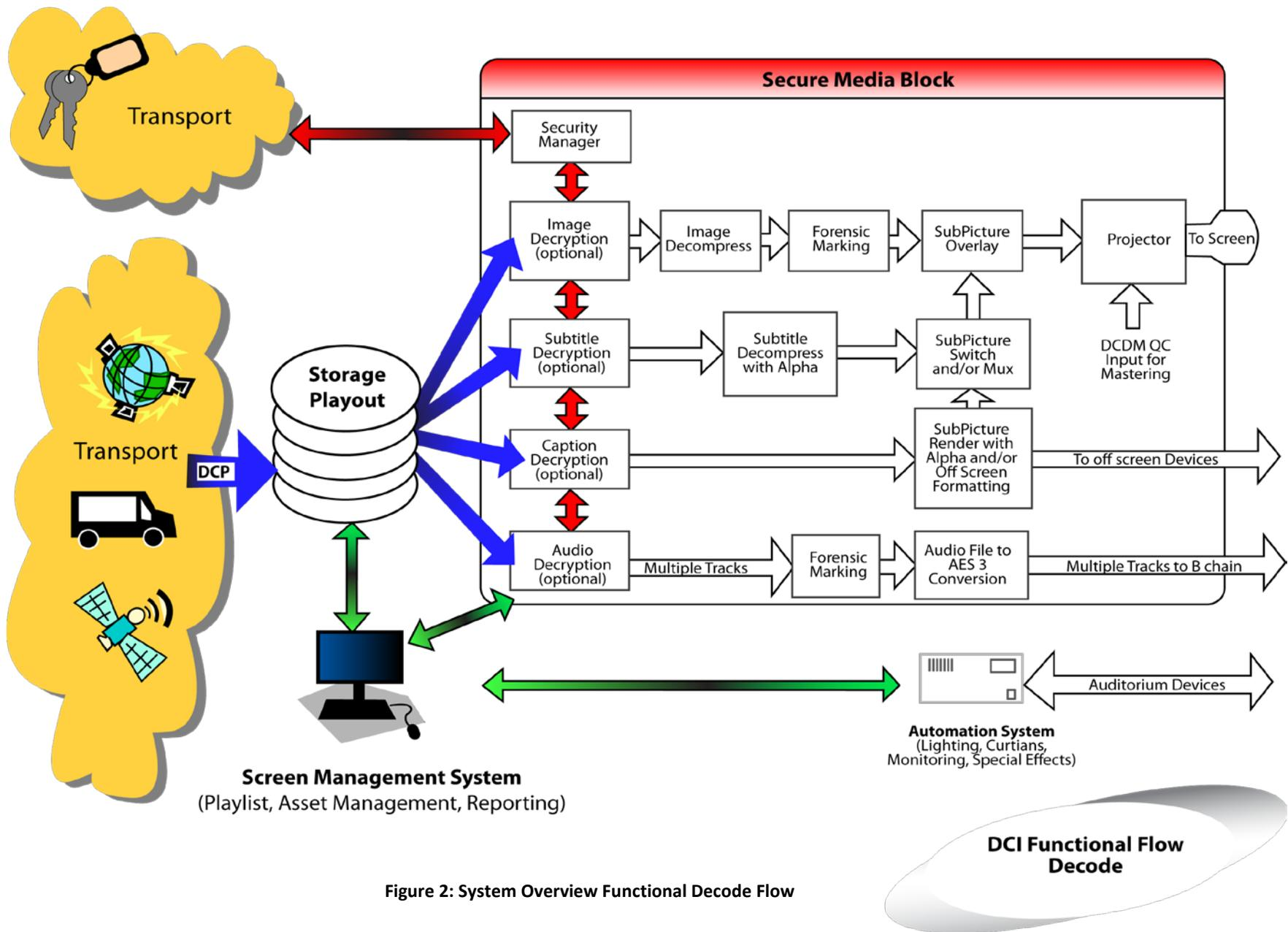
Figure 2: System Overview Functional Decode Flow
