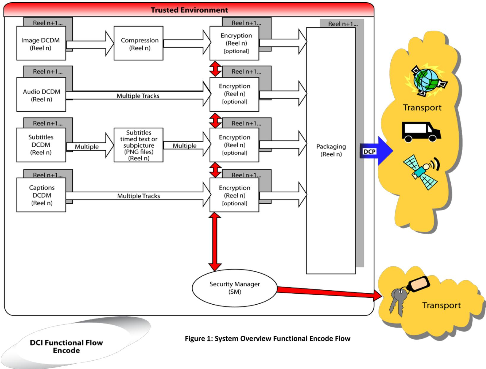
Figure 1: System Overview Functional Encode Flow
